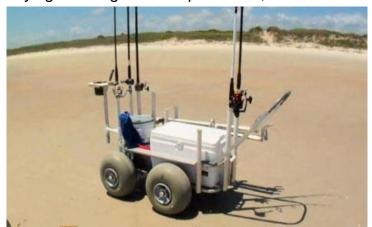
Also in the overall size is the carrying capacity of it, and that it be made of a lightweight rustproof or rust-resistant material like aluminium or PVC. The wheels should be wide enough that they won't sink into the soft sand, golf cart wheels or balloon tyres are ideal for this purpose, although stay away from any with tubes or bearings, bushes only, there's no roadside assist here if you get a flat.
